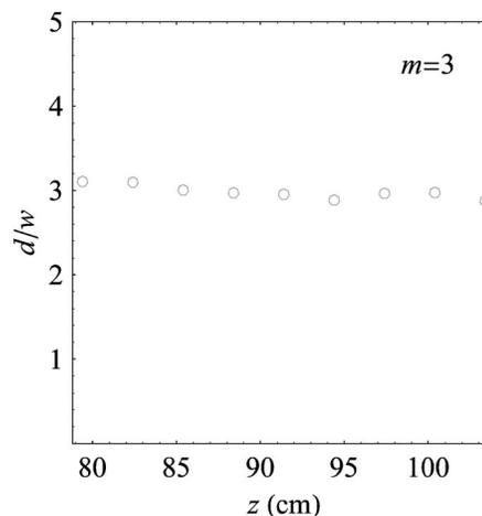
Fig. 3. Ratio between the diameter  $d(z)$  of the  $|\text{HyGG}\rangle_{-3,3}$  mode and the  $1/e^2$  intensity radius  $w(z)$  of the generating TEM<sub>00</sub> Gaussian beam as a function of  $z$ . The Rayleigh range was  $z_0 = 7.8$  cm.
