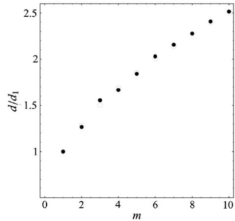
Fig. 2. Ring diameter  $d$  of the  $|\text{HyGG}\rangle_{-m,m}$  mode for  $m=1, \dots, 10$  measured at plane  $z=0.18z_0$ . The Rayleigh range was  $z_0=747.4$  cm. The reported values of the diameters were scaled with respect to the value  $d_1$  for  $m=1$ .  $\circ$ , theory;  $\bullet$ , experiment.
