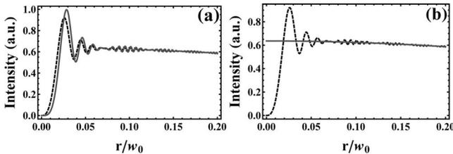
Fig. 2. Intensity profile for (a) full STOC and (b) no STOC in the 1-plate. Solid and dashed curves are simulated by [7] and our theory, respectively. The input beam assumed the  $TEM_{00}$ .
