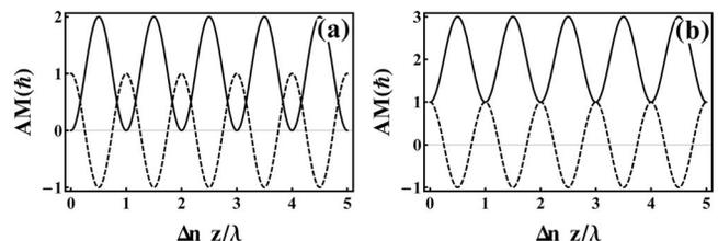
Fig. 1. Beating of SAM (dashed curve) and OAM (solid curve) as a function of the optical retardation  $\Delta n z/\lambda$  while a circularly polarized input beam propagates in the 1-plate. (a) For  $\text{LG}_{00}$  and (b)  $\text{LG}_{01}$  as an input beam. We used the following data:  $n_o = 1.5$ ,  $n_e = 1.7$ , and  $w_0 = 50\lambda$ .
