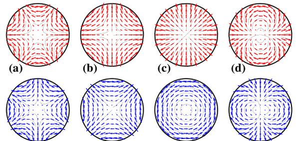
FIG. 1 (color online). Electric (upper panels) and magnetic (lower panels) field  $q$ -filter geometries for different topological charges: (a)  $q = -2$ , (b)  $q = -1$ , (c)  $q = 1$ , and (d)  $q = +2$ ; in all cases,  $\beta = \pi/2$ .
