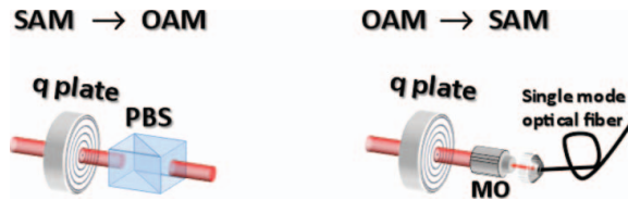
Figure 4. Pictorial representation of the simplest non-unitary (probabilistic) devices for the transfer of a qubit of quantum information from the polarization to the OAM ( \text{SAM} \rightarrow \text{OAM} ) and vice versa ( \text{OAM} \rightarrow \text{SAM} ) [22, 29]. The first is based on a q-plate and a polarizing beam splitter (PBS). The second requires a q-plate and a zero-OAM-filter, as obtained by coupling into a single mode fiber (using a microscope objective, MO).
