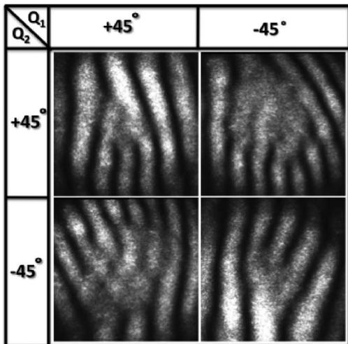
Fig. 4. The interference of the output beam from the loop device and TEM<sub>00</sub> beam for the four QWP angles shown in Table 1.
