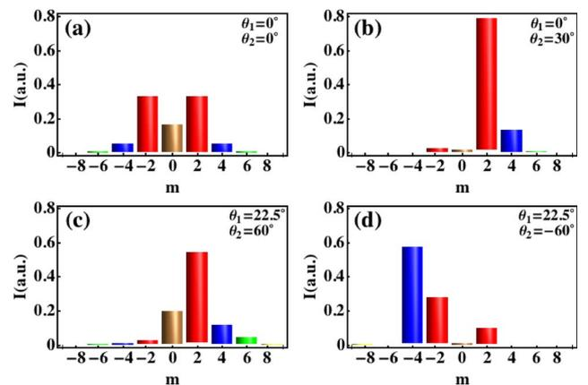
Fig. 3. (Color online) Calculated OAM power spectrum  $I_n = |c_{2n}|^2$  of the beam emerging from the loop device for different angles  $\theta_1$  and  $\theta_2$  of the two QWPs for loop delay  $\psi = 0$ . The power spectrum can be either (a) symmetric or (b), (c), (d) not symmetric, and (b), (d) the fundamental  $m = 0$  component can be suppressed.
