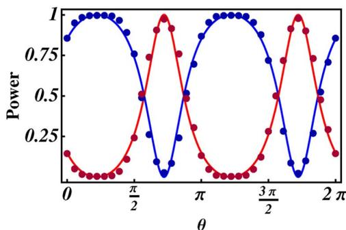
Fig. 5. (Color online) The normalized powers of the  $m = 2$  (blue) and  $m = -4$  (red) components of the loop output beam as functions of the orientation angle  $\theta$  of the second QWP. The first QWP was held fixed at  $45^\circ$ . The continuous curve is the fit to the square moduli of the coefficients of modes  $m = 2$  and  $m = -4$  in Eq. (5). The optical retardation  $\psi$  of the loop was used as fitting parameter. In this case, we found a best-fit value  $\psi = 0$ .
